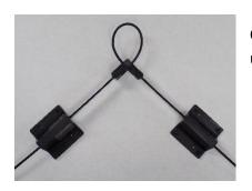
Crack Sensor: Measure movement of identified crack. Can be done up to a three-axis movement.
